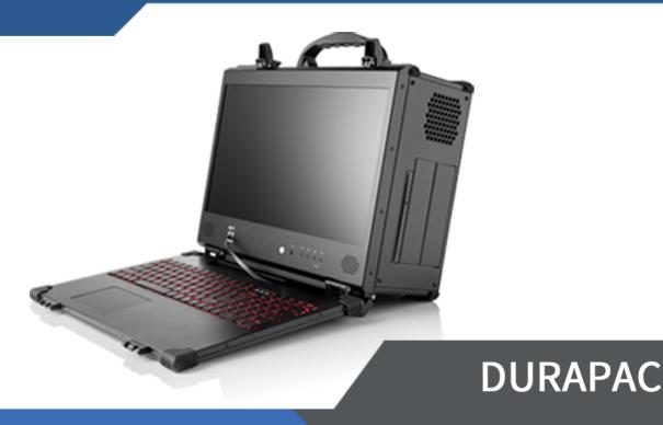
The DuraPAC product is a robust portable computer built using all aluminum sheet metal to provide tough, go-anywhere unit suitable for tough environments and mobile applications. With the 17.3", HD LCD display and 4-expansion slots design, the DuraPAC can easily fulfill the requirements for many applications including digital media and broadcasting.
