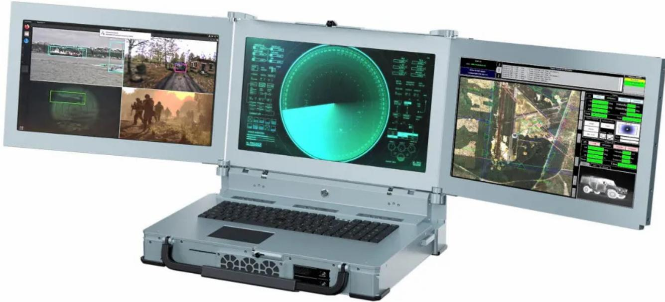
High-performance rugged laptop with server-grade performance and three tiltable 17.3" full HD displays.
